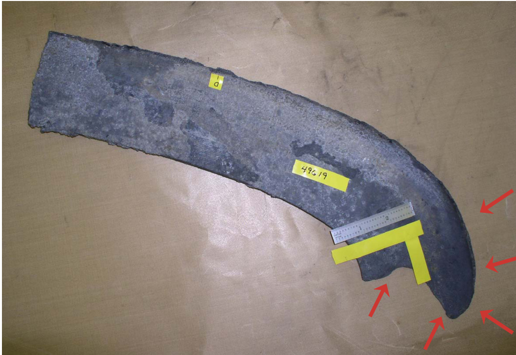
Figure 4.—Recovered portion of panel 8L, showing knife edge.
