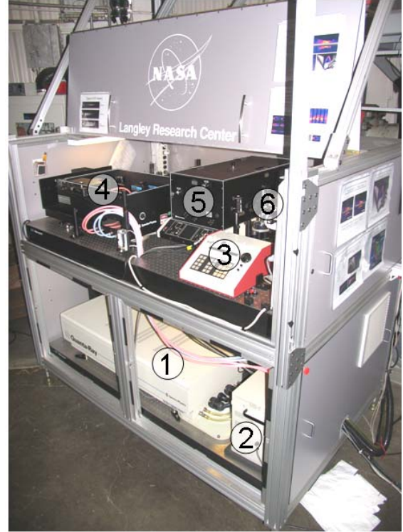
Figure 3. The portable PLIF system. Here, the system is shown with panels removed. Components include: (1) Nd:YAG laser; (2) dye circulators with Rhodamine 590 and Rhodamine 610 laser dyes in a methanol solvent; (3) wavelength controller for the (4) pulsed dye laser; (5) wavelength extender; and (6) low pressure monitoring gas cell.
