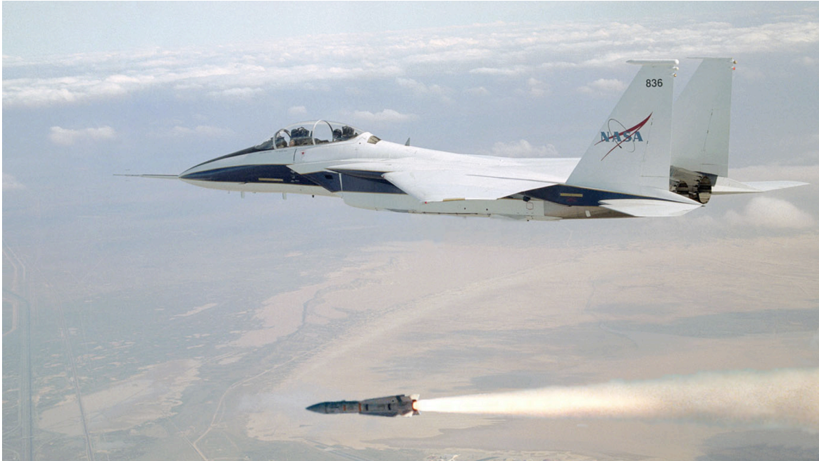
Figure 2. Computer-enhanced photograph of the proposed ALSM hypersonic test and evaluation platform.
