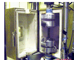
Figure 3. ASTM D3165 Lap Shear Specimen and Oven Test Configuration
