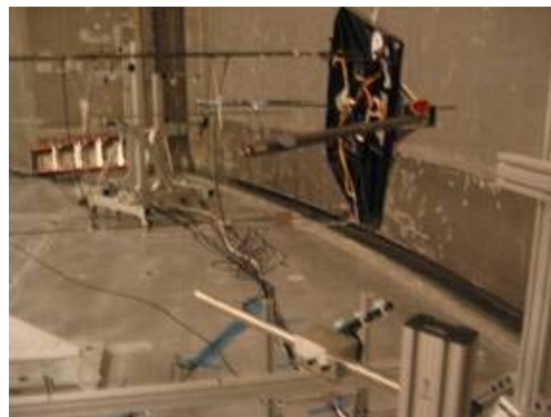
Figure 14. Spreader Bar at Mast Tip
