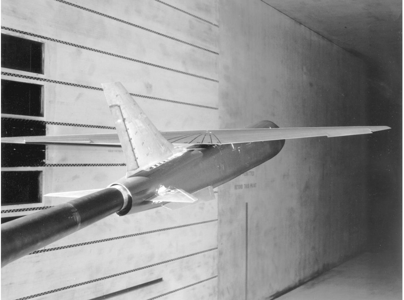
Figure 5(b). Installation photograph of the F-8 OWRA model with Ames 300 sq ft wing.
