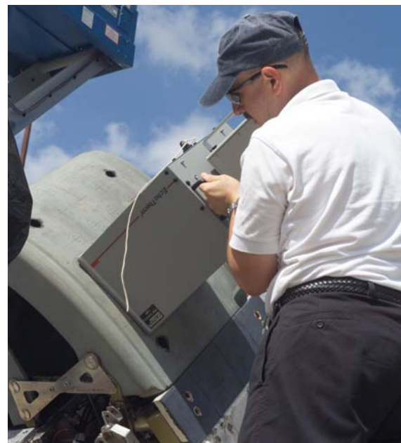
Figure 8. Photograph of thermographic inspection of RCC test panel after impact testing.
