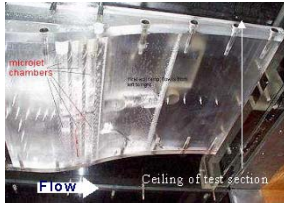
Fig. 1- Ramp model, mounted in the wind tunnel
