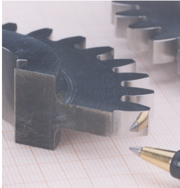
Figure 4.2.4.—Near-mirror quality of superfinished tooth surface.
