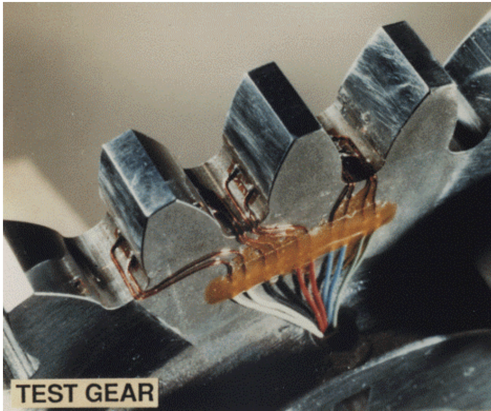
Figure 5.2.1.—Test gear instrumented with strain gages on both sides of successive teeth.
