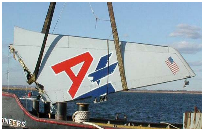
Figure 4: Vertical stabilizer as recovered from Jamaica Bay.
