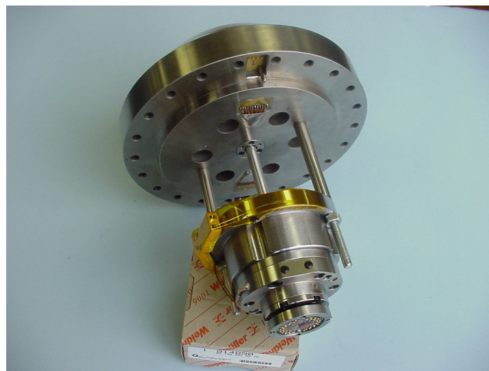
Figure 4.5.3-1.—Test rig arbor and slip ring bearing sub-assembly.
