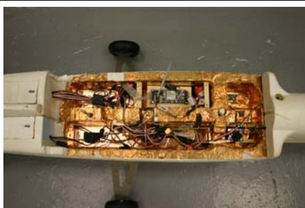
Figure 6. Interior bay of NASA modified Army FQM-117B UAV.
