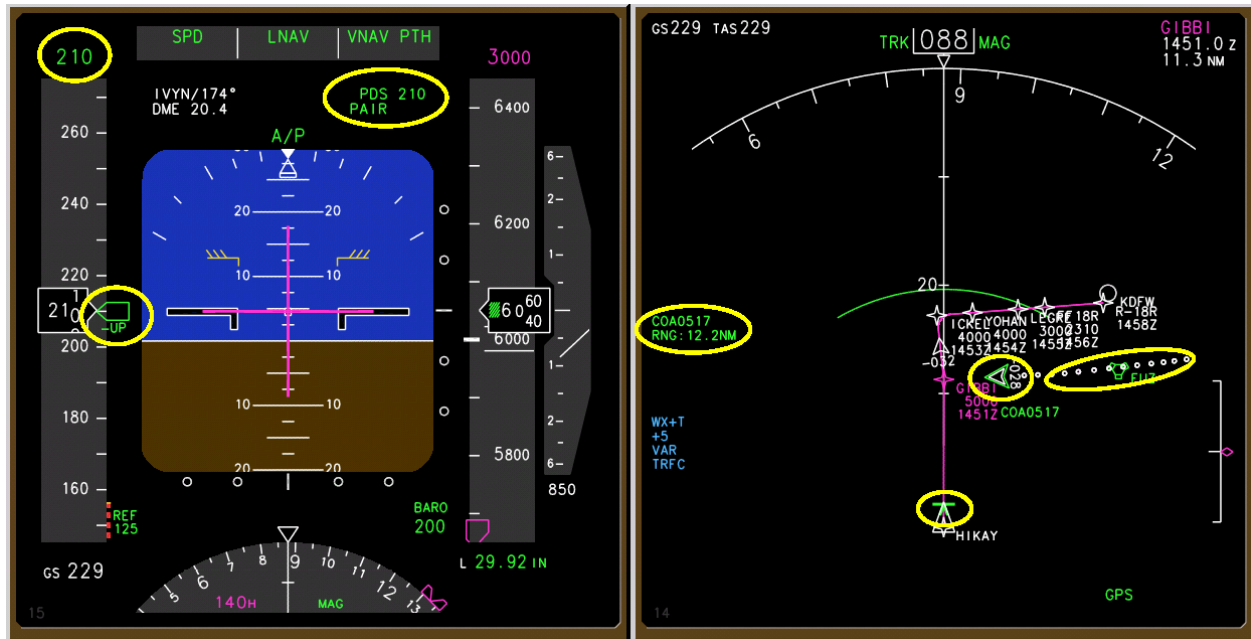
Figure 5. The ASTOR Primary Flight Display (PFD) and Navigation Display (ND). All new symbology is circled in yellow: on the PFD this includes the green text in the upper right and the green speed target and speed bug; on the ND it includes the spacing position indicator just in front of the ownship, the highlighted lead aircraft, the history dots for the lead aircraft and the text block on the left hand side.
