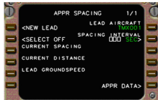
Figure 4. The ASTOR Multi-function Control Display Unit (MCDU) showing the input page for AMSTAR.
