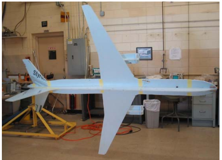
Figure 10. 5.5% GTM-ADM undergoing pitch testing
