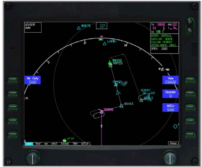
Figure 1. HVO MFD (white own-ship, traffic to follow double-blue chevron, green “Entry” message, solid line instrument approach, dotted line missed approach)
