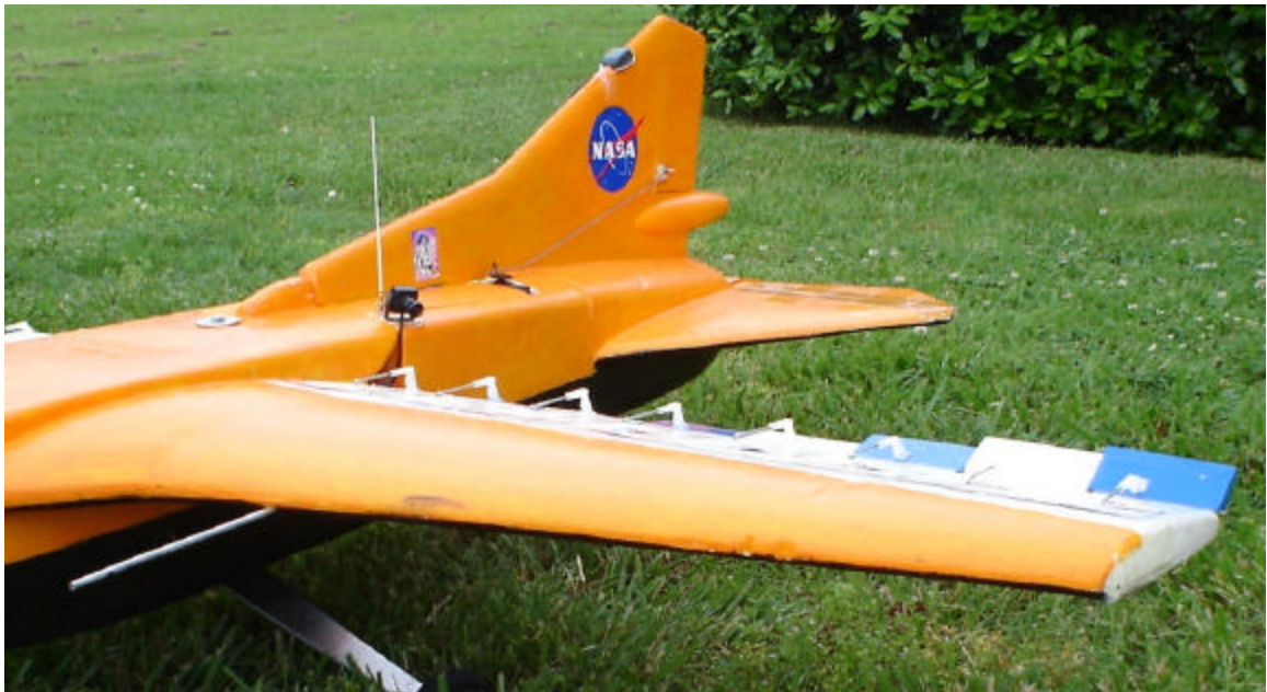
Figure 3. FLiC configured with 16 Aileron Segments
