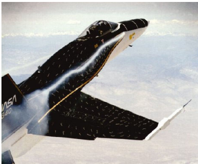
Figure 1. Vortices from the leading edge of a twin-tail fighter aircraft, generated at high angles of attack, breakdown upstream of the empennage.
