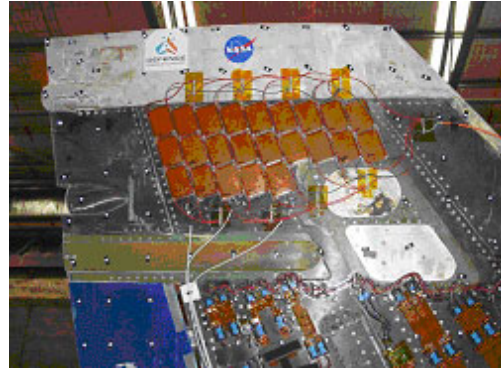
Figure 8. NASA LaRC MFC actuators installed on F/A-18 (ST01) in preparation for ground testing.
