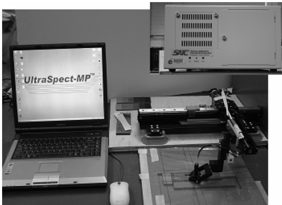
Figure 2. SAIC Ultraspect-MP eddy system for in-situ eddy current inspections of RCC.
