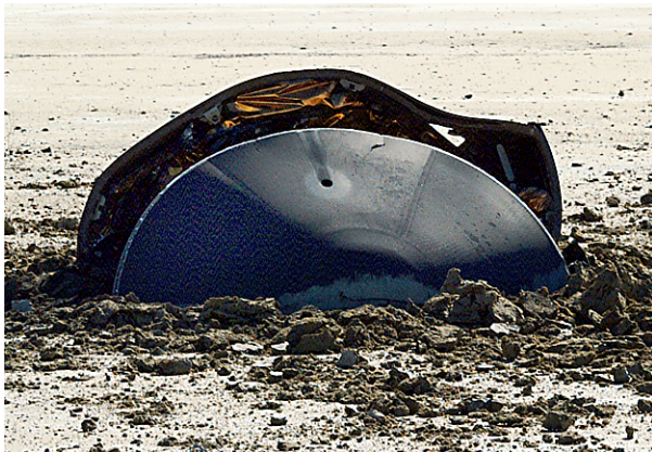
Fig. 13. Image of capsule forebody heatshield
