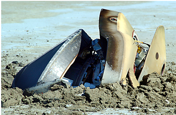
Fig. 12. Image of capsule shoulder region and aftbody heatshield
