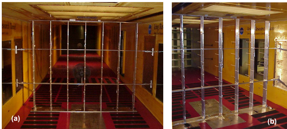
Figure 5. Installation of the 2-D RTD Array in the IRT test section. (a) view looking downstream. (b) view looking upstream.
