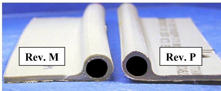
Figure 4.—Photograph comparing as-received Rev. P seal to as-received Rev. M seal. Note the presence of Nomex fabric impregnation of Rev. M seal bulb.
