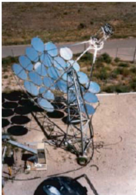
Figure 7.—A 5-kilowatt point-focus Stirling engine concentrator system (courtesy of Cummins Power Generation, Inc.).
