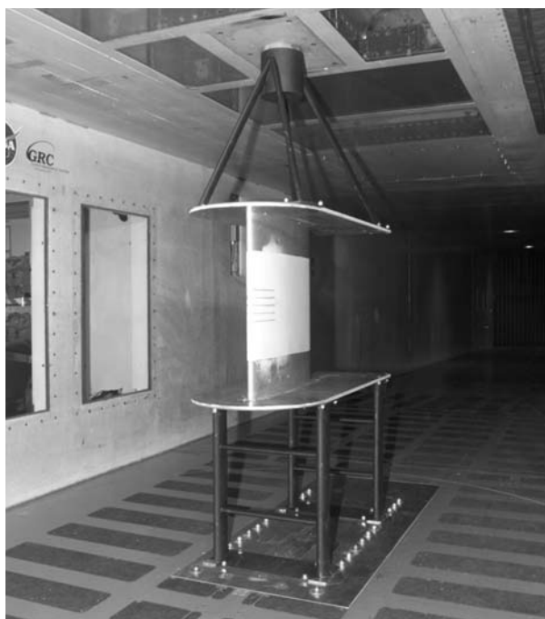
(b) 53.3-cm-Chord NACA 0012 Model Installed in IRT Test Section.
