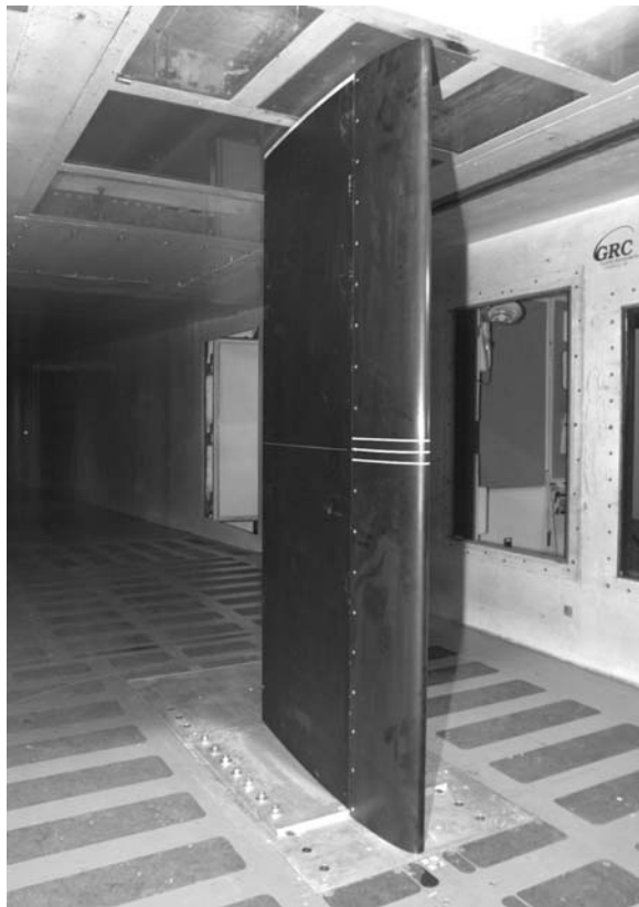
(a) 91.4-cm-Chord NACA 0012 Model Installed in IRT Test Section.
