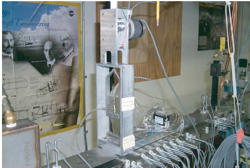
Figure 4. Photograph of 9-Probe Flow Measurement System.
