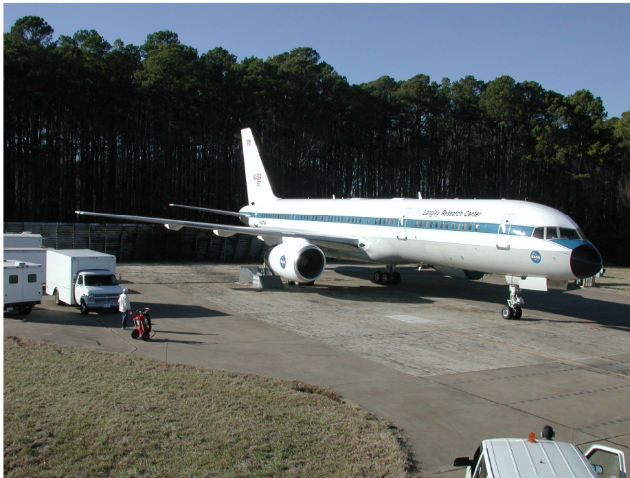
Figure 5. Photograph of experimental setup showing B-757 with the sampling stand positioned behind right engine and equipment trailers parked off right wing.
