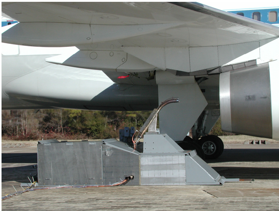
Figure 4. Photograph of sampling sled and instrument container positioned behind the right engine of B-757.
