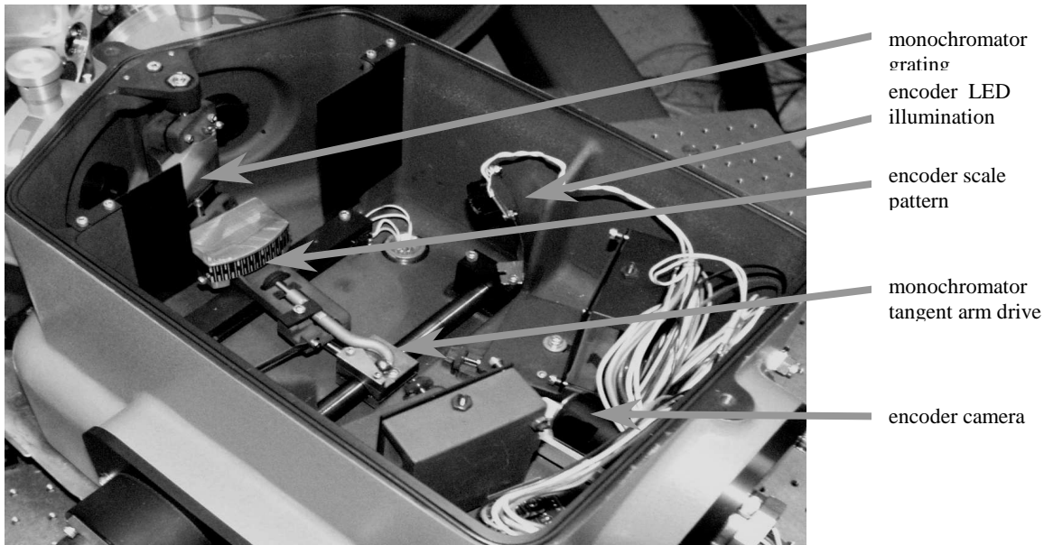
Figure 3: Absolute optical encoder adapted to report shaft angle of grating inside vacuum monochromator
