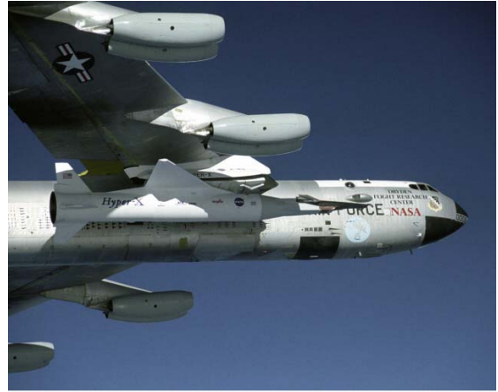
Figure 5 Hyper-X stack being carried to altitude on the NASA B-52B
