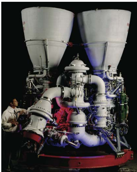
Figure 3. Pratt & Whitney RD-180 engine (image courtesy of Pratt & Whitney).
