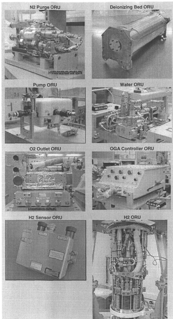
Figure 8. Oxygen Generation Assembly Flight Hardware
