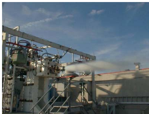
Figure 11. Subscale oxygen-rich preburner hotfire testing at E-2 test stand. Oxygen rich mixture ratio results in a white color plume at relatively low temperature.
