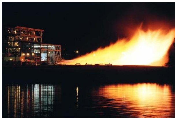
Figure 9. IPD fuel pump cold-flow test at SSC E-1 stand (Cell 2); the high flow of gaseous hydrogen efflux is flared in front of the test cell upon exhaust by using exit igniters whereas the liquid hydrogen is disposed to the high pressure flarestack behind the test stand (not shown).
