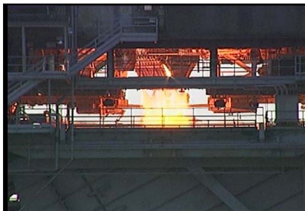
Figure 5. Aerospike dual-engine hotfire test at A-1 test stand at SSC. The J-deflector flame bucket, below the engine deck, turns to the right in the picture to direct the flame.
