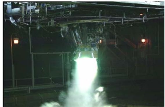
Figure 2. Hotfire testing of the MC-1 64 Klbf LOX/kerosene engine with its battleship stage installed vertically in the test stand (stage aft end is visible above the engine).
