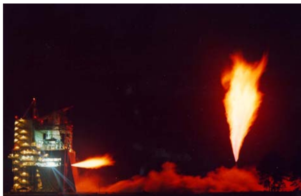
Figure 4. Panoramic view of powerpack hotfire test at A-1 test stand at SSC. The gas generator exhaust is seen at left, and hydrogen burnoff through a facility flarestack at right, in picture.
