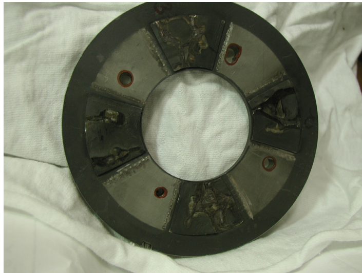
Figure 8.—Post-test photograph of the modified foil thrust bearing.
