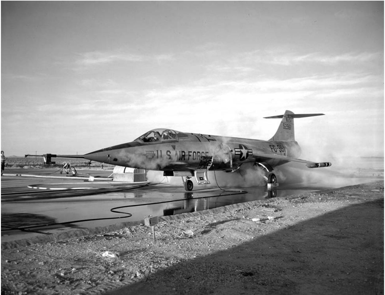
Figure 25. Testing the F-104 reaction control system at Edwards Air Force Base, December, 1960.
