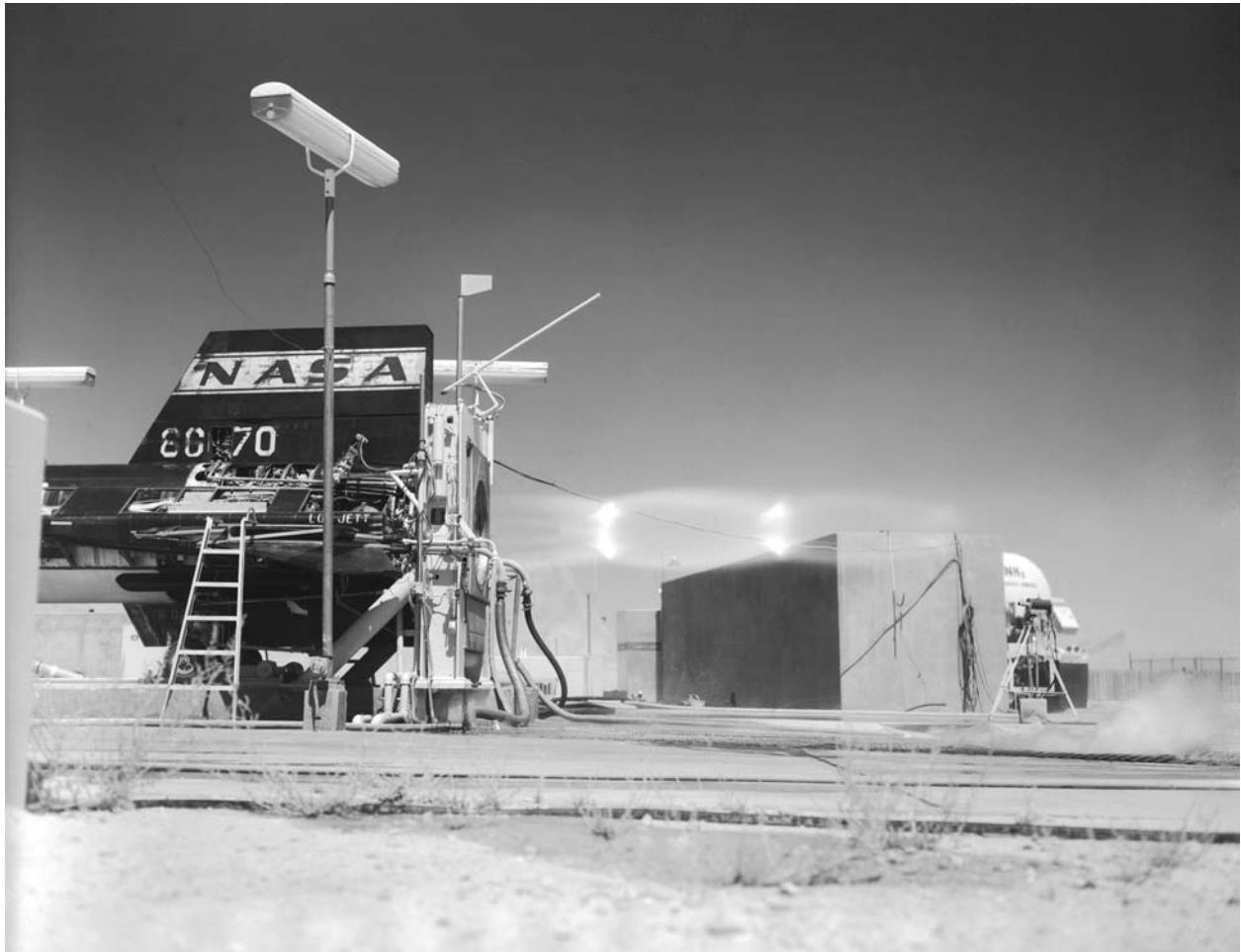
Figure 23. The X-15 rocket-powered research airplane with the XLR-99 rocket engine configuration during testing on the south test stand.
