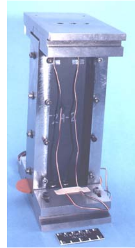
a) Impact panel prior to testing.
