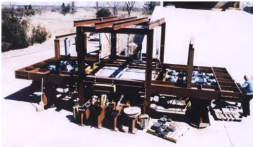
Figure 13. Photograph of pressure-box test fixture.
