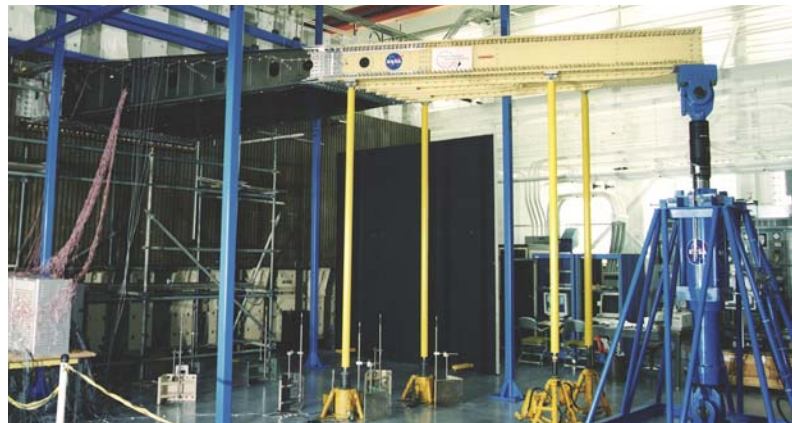
Figure 8. Wing stub box prior to testing.
