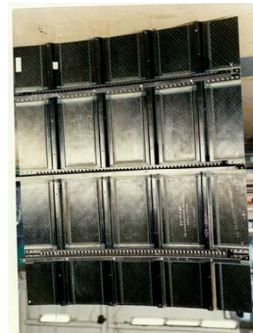
Figure 12. Photograph of a typical benchmark crown panel.
