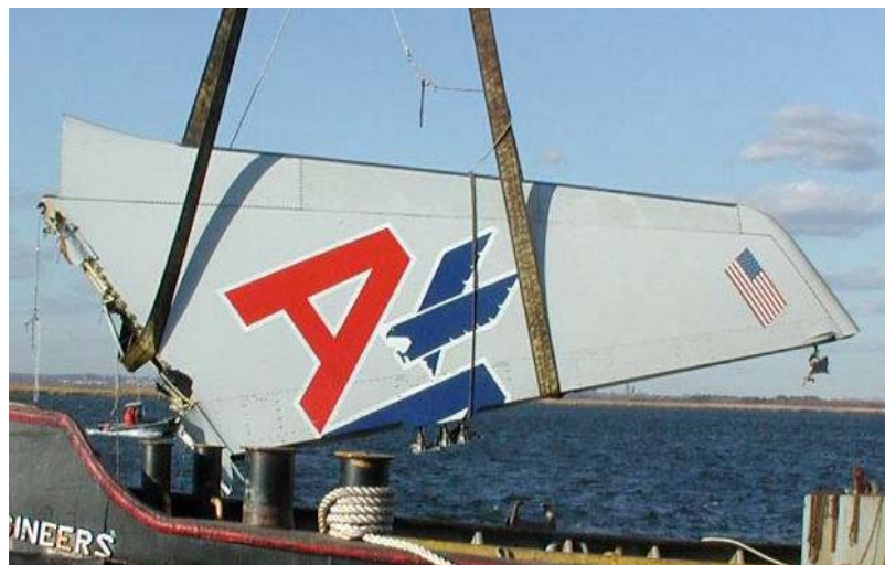
Figure 3. Vertical stabilizer as recovered from Jamaica Bay.
