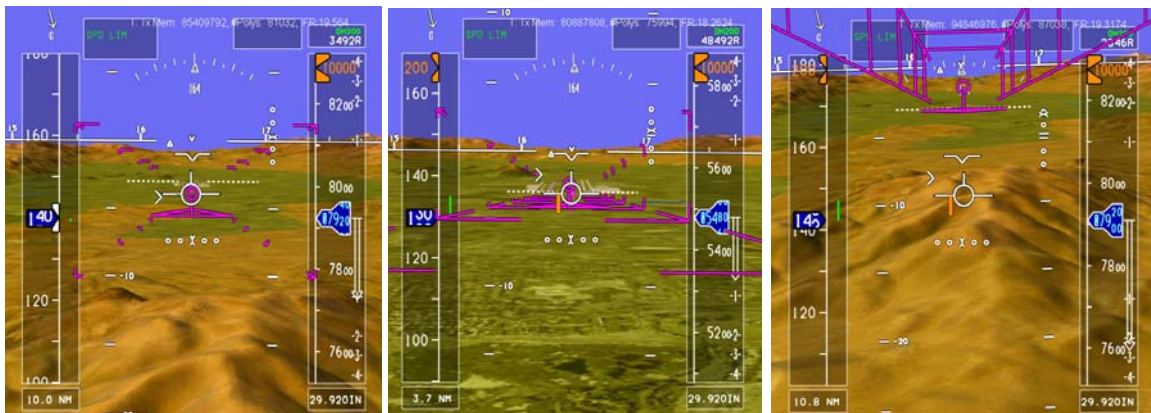
Figure 6. Dynamic Pathway-In-The-Sky Tunnel
