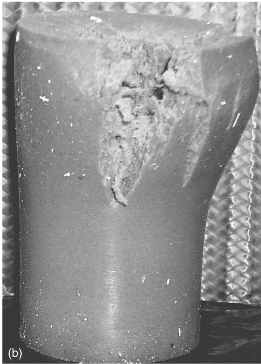
Fig. 3. Gelatin projectile. (a) Before impact. (b) After impact.
