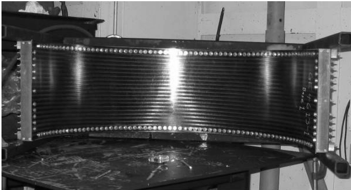
Fig. 5. Test fixtures for the 112 cm (44 in.) diameter composite half-rings.
