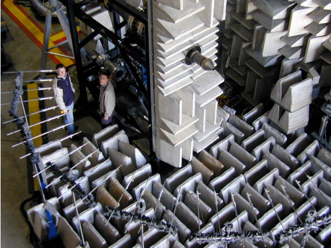
Figure 1 Small Hot Jet Acoustic Rig with microphone array.
