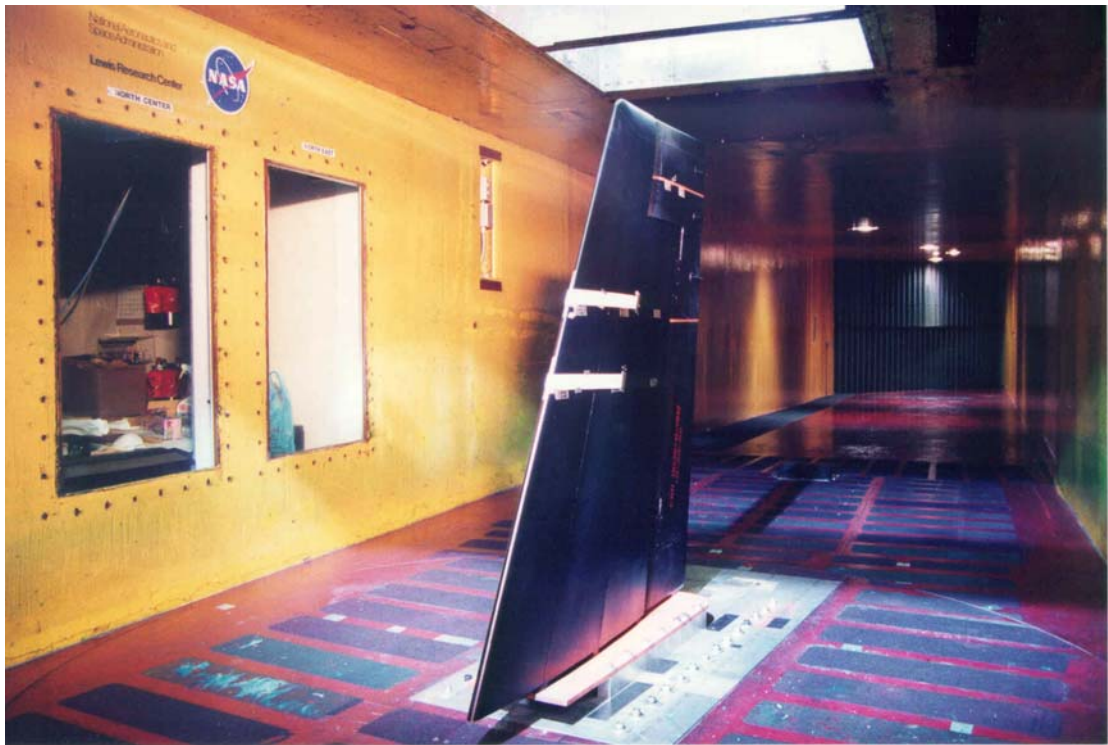
Figure 4: Illustration of wing blotter strip installation.
