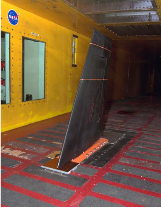
(a) Installation in IRT.
