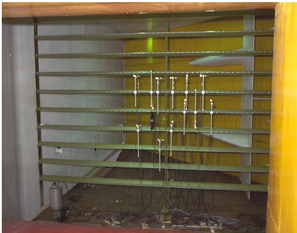
Figure 2: Installation of spray system used for Icing Research Tunnel impingement tests.
