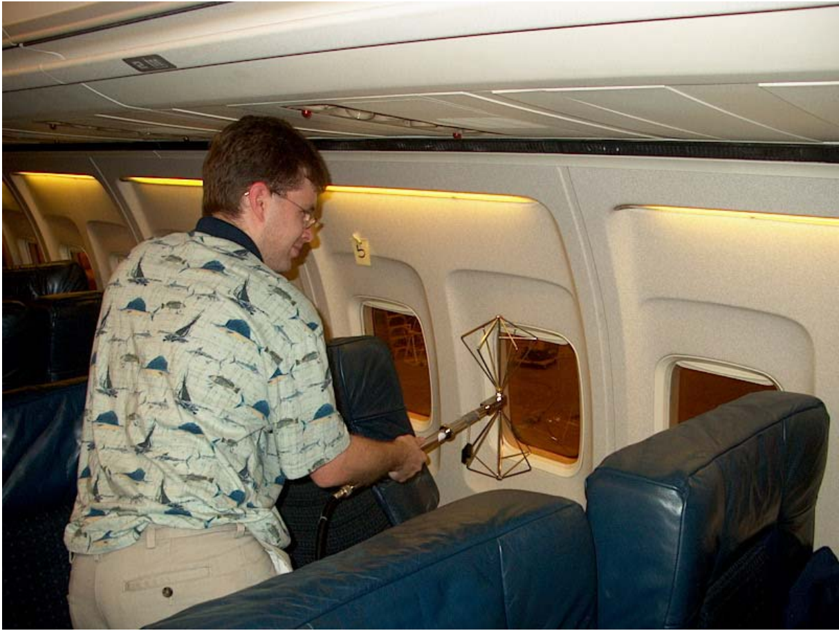
Figure 7 – 690 IPL Measurement Using Bicon Antenna
