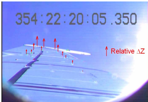
Figure 9: Relative Z -deflection overlaid on video image of wing.
