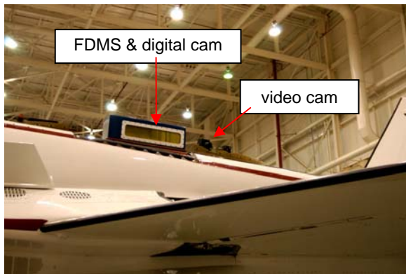
Figure 6: Camera locations on F/A-18.
