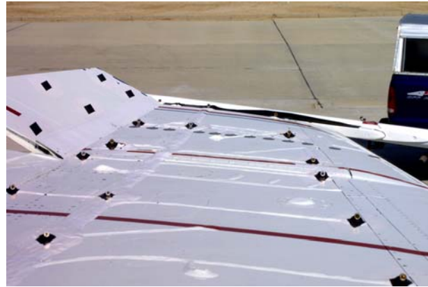
Figure 17: Black diamond targets on AAW F/A-18.
