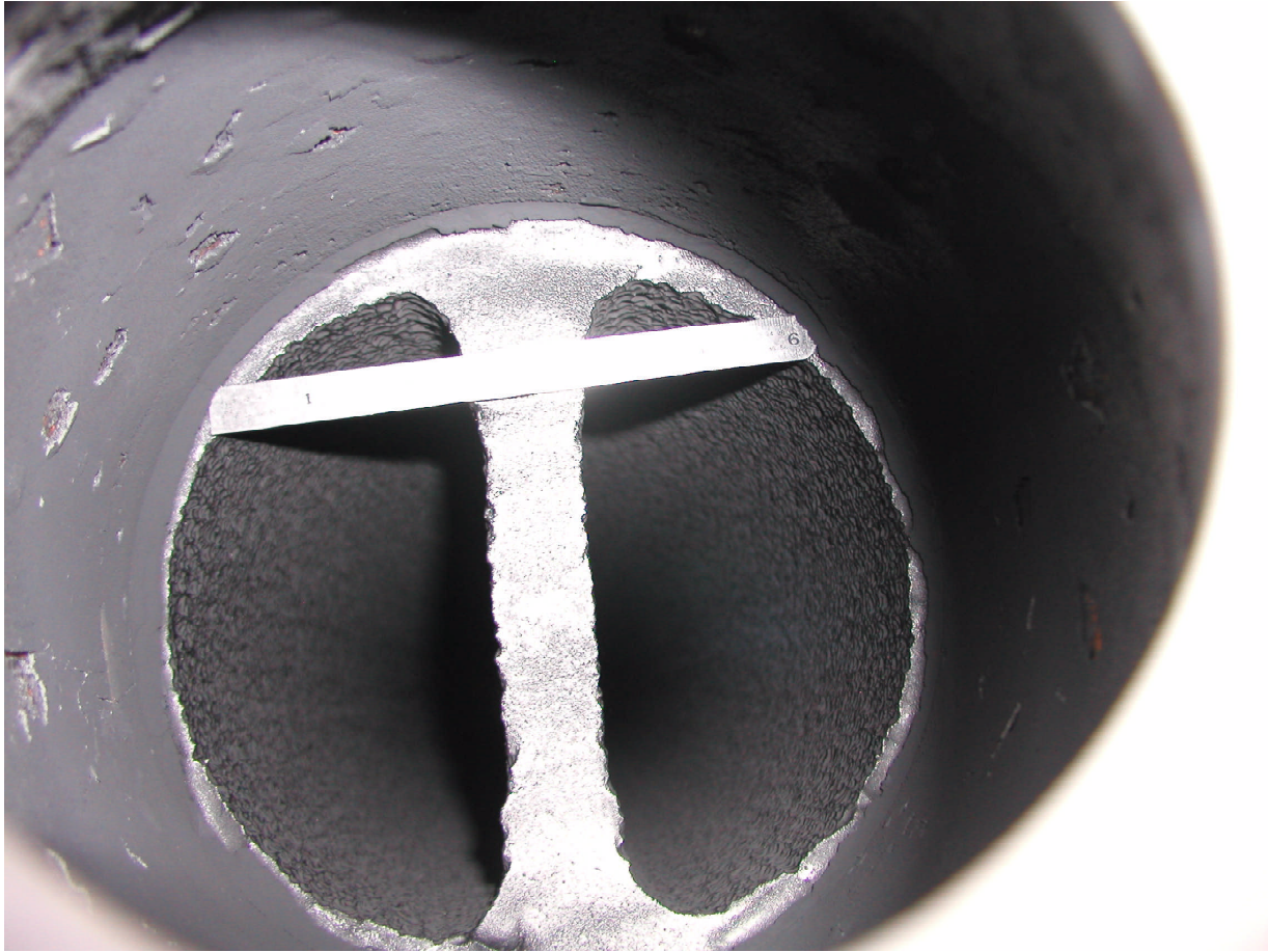
Figure 7 – The HTT-02 Post Test fuel grain as viewed through the nozzle
