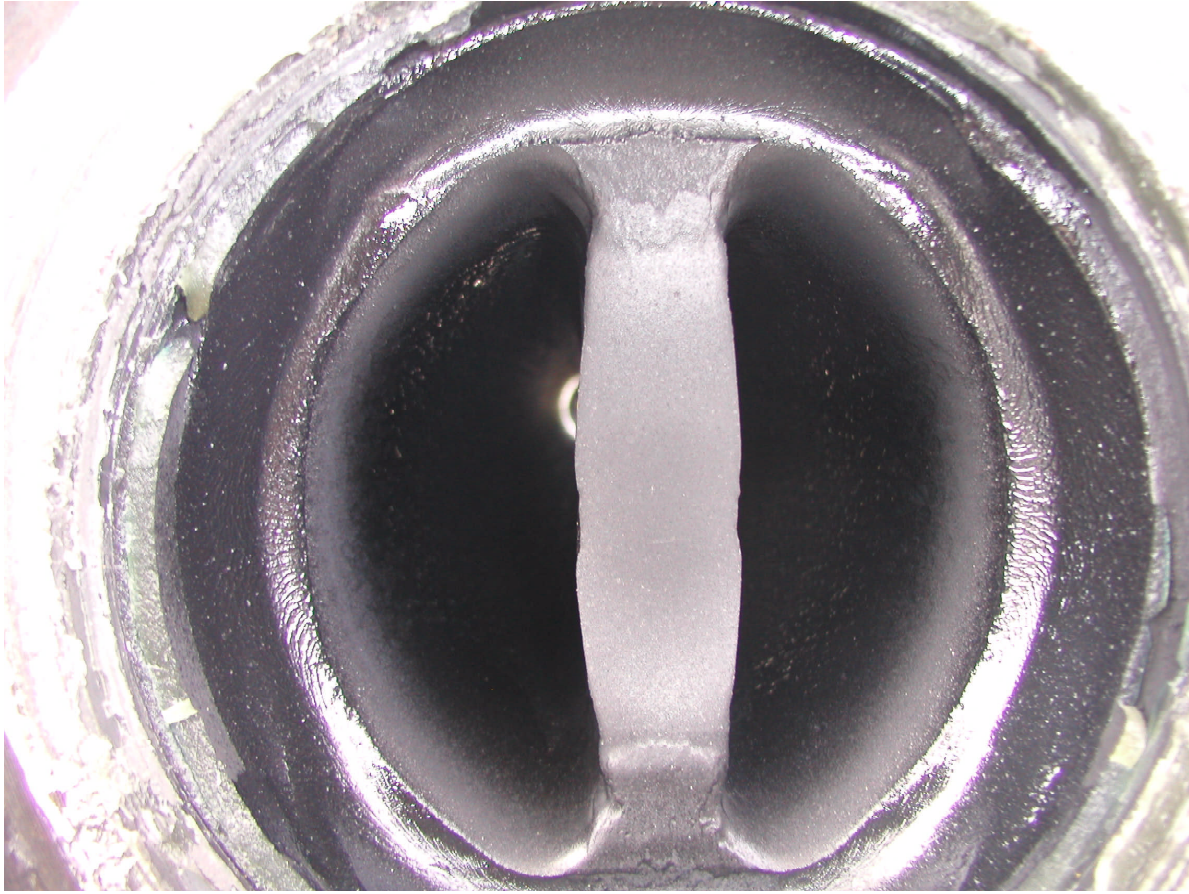
Figure 8 – The HTT-02 Post Test fuel grain as through the head end
