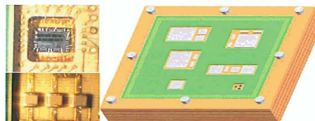
MSFC Model of Stacked Substrate Embedded Component (solderless box-less cube) 400-600% size reduction
