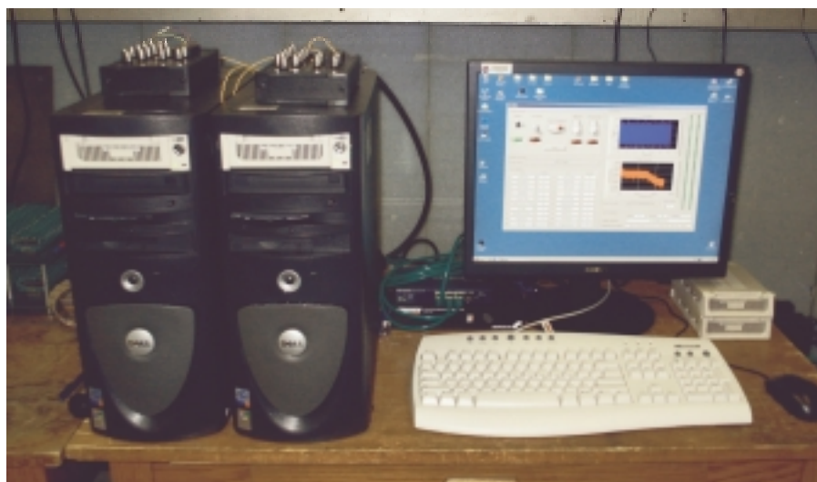
Figure 7. Distributed (Two-Node) Data Acquisition System.
