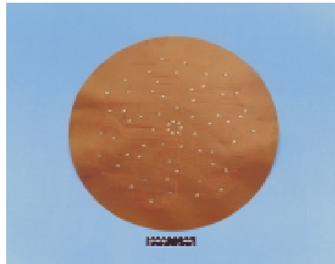
Figure 3. Prototype Kapton Sheet Containing 63 MEMS Microphones.
