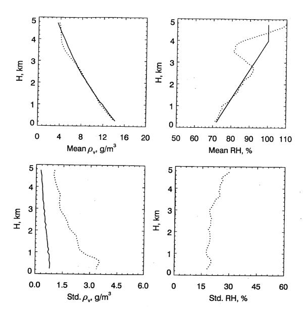
Fig.13. Top left: Mean profiles of estimated (dashed line) and assumed (solid) water vapor density versus height. Top right: Mean profiles of estimated (dashed line) and assumed (solid) relative humidity, RH. Bottom left: Standard deviation of estimated (dashed line) and assumed (solid) water vapor density. Bottom right: Standard deviation of estimated (dashed line) relative humidity. n=16,000 and 20% bandwidth.
