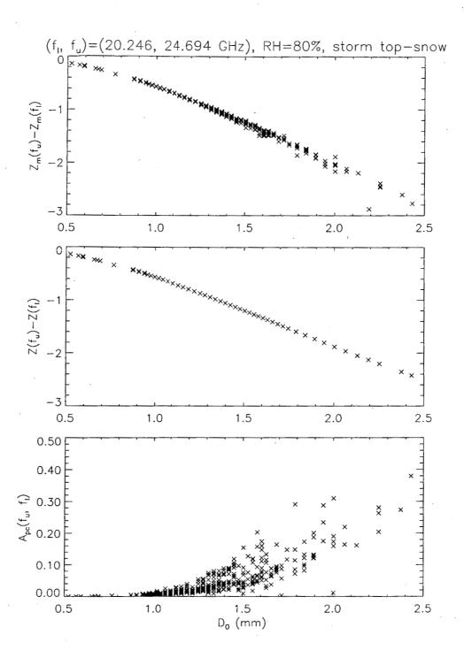
Fig.5. Measured (top) and 'actual' (center) differential reflectivity factor and differential path attenuation (bottom) for a range gate in the snow just above the melting layer versus median drop diameter of melted particles, D<sub>0</sub>.
