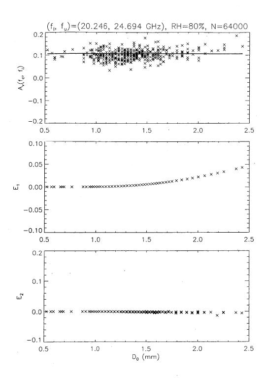
Fig.6. Top: Assumed (solid line) and estimated differential water vapor absorption (X) in snow versus median drop diameter of melted particles; Center: Bias term  $E_1$ ; Bottom: Bias term  $E_2$ .  $\gamma$ =0.42.
