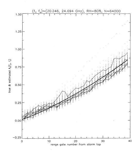
Fig.8. Five profiles of estimated differential water vapor absorption (thin lines) and assumed differential absorption (thick line) versus range gate number from storm top. The range gate spacing is 125 m. Results from all estimated profiles are indicated by the '+" symbol.
