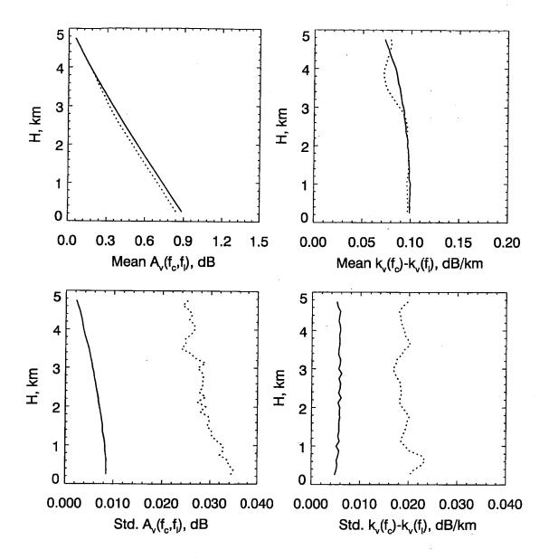
Fig. 12. Top left: Mean profiles of estimated (dashed line) and assumed (solid) differential water vapor attenuation versus height. Top right: Mean profiles of estimated (dashed line) and assumed (solid) differential specific attenuation. Bottom left: Standard deviation of estimated (dashed line) and assumed (solid) differential water vapor attenuation. Bottom right: Standard deviation of estimated (dashed line) and assumed specific differential attenuation. n=16,000 and 20% bandwidth.
