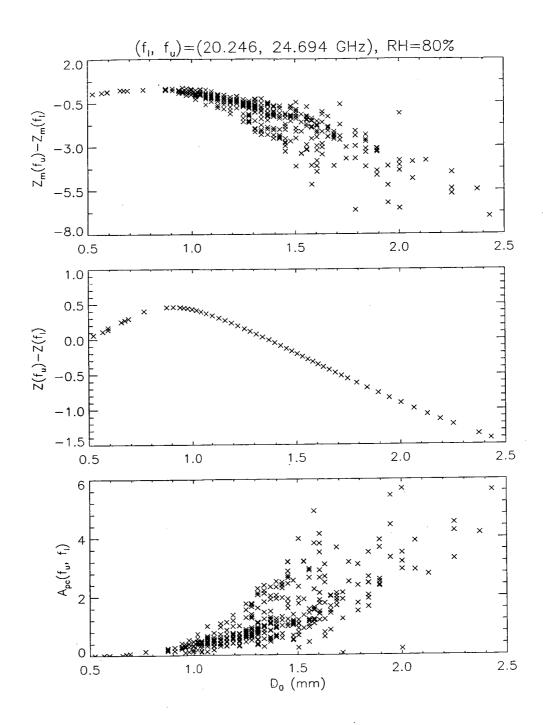
Fig.3. Measured (top) and actual (center) differential reflectivity factor and differential path attenuation from precipitation (bottom) for a range gate near the surface versus the median drop diameter,  $D_0$ . All units are in dB.
