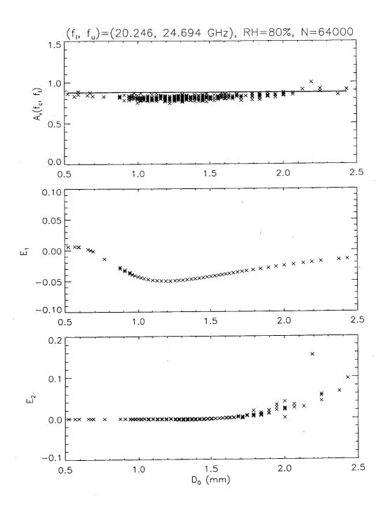
Fig.4. Top: Assumed (solid line) and estimated differential water vapor absorption (X) versus median raindrop diameter for a range gate near the surface; Center: Bias term  $E_1$ ; Bottom: Bias term  $E_2$  versus median drop diameter.  $\gamma$ =0.42.
