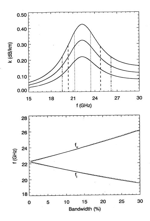
Fig.1. Top: Specific absorption of water vapor (dB/km) for water vapor densities (g/m³) of 8.75 (lowest), 13.15, 17.5 (highest) and the frequencies at which the absorption is equal for bandwidths of 10%, 20% and 30%. Bottom: Upper and lower frequencies giving equal water vapor absorptions versus percent bandwidth. Solid lines represent numerical values; dashed lines represent quadratic approximations given by (8) and (9).
