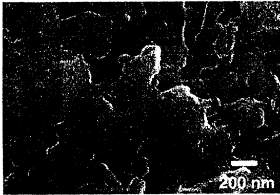
Figure 6. Fracture cross-section of oxide grown on AlN at 1200°C for 100h in dry oxygen (left) and for 48h in wet oxygen (right).
