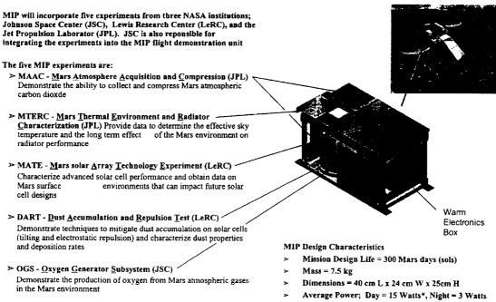
\* When producing oxygen; 9 Watts average without oxygen production
