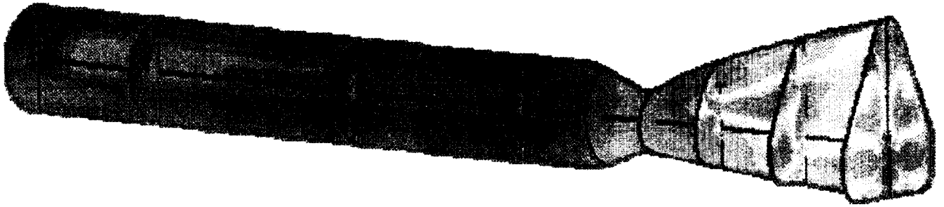
Figure 9a: Combined Cycle 3d analysis, contour plot of mach number.
