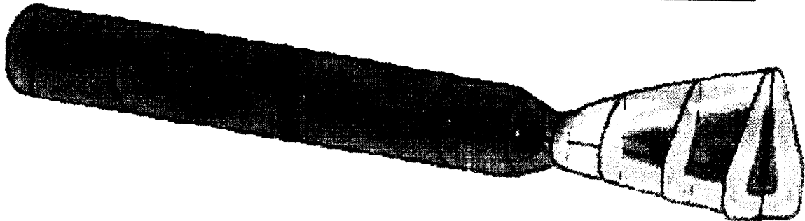
Figure 9e: Combined Cycle 3d analysis, contour plot of H 2 mass fraction.
