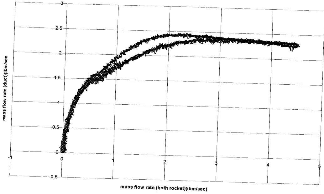
Figure 9. Mass Flow of Duct Compared to Mass Flow of both Rockets
