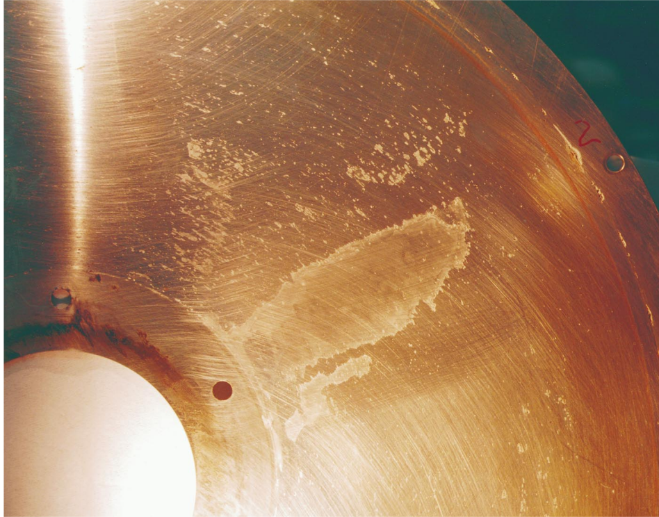
Figure 37. VCD-5A end plate showing light corrosion.
