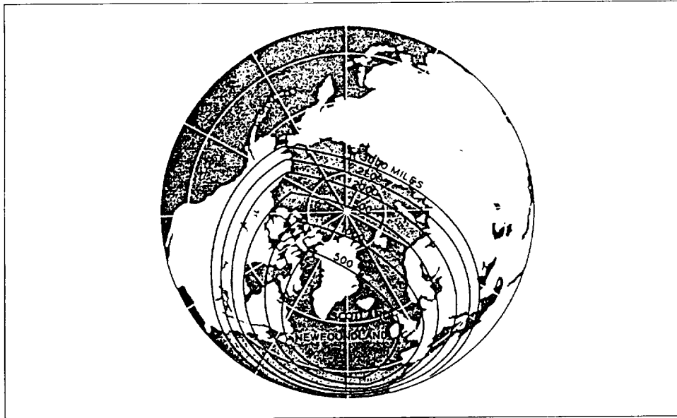
Oval-shaped areas define regions in which polar-orbit satellites at various heights would be simultaneously visible to both terminals at Newfoundland and Scotland. The usable areas would be somewhat smaller, however, since transmission is difficult when [the] satellite is near the horizon.
